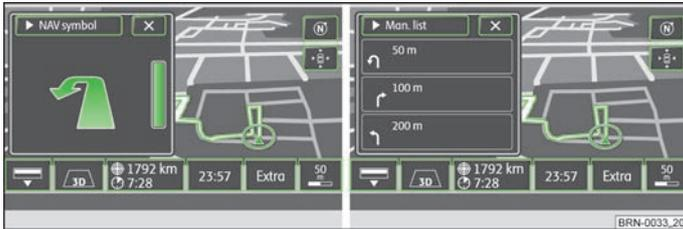
Fig. 12 Split-screen displaying the navigation information/split-screen displaying the information list
